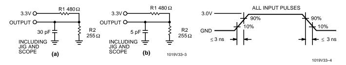
Equivalent to: THÉVENIN EQUIVALENT <u>167Ω</u> OUTPUT O -0 1.73V
